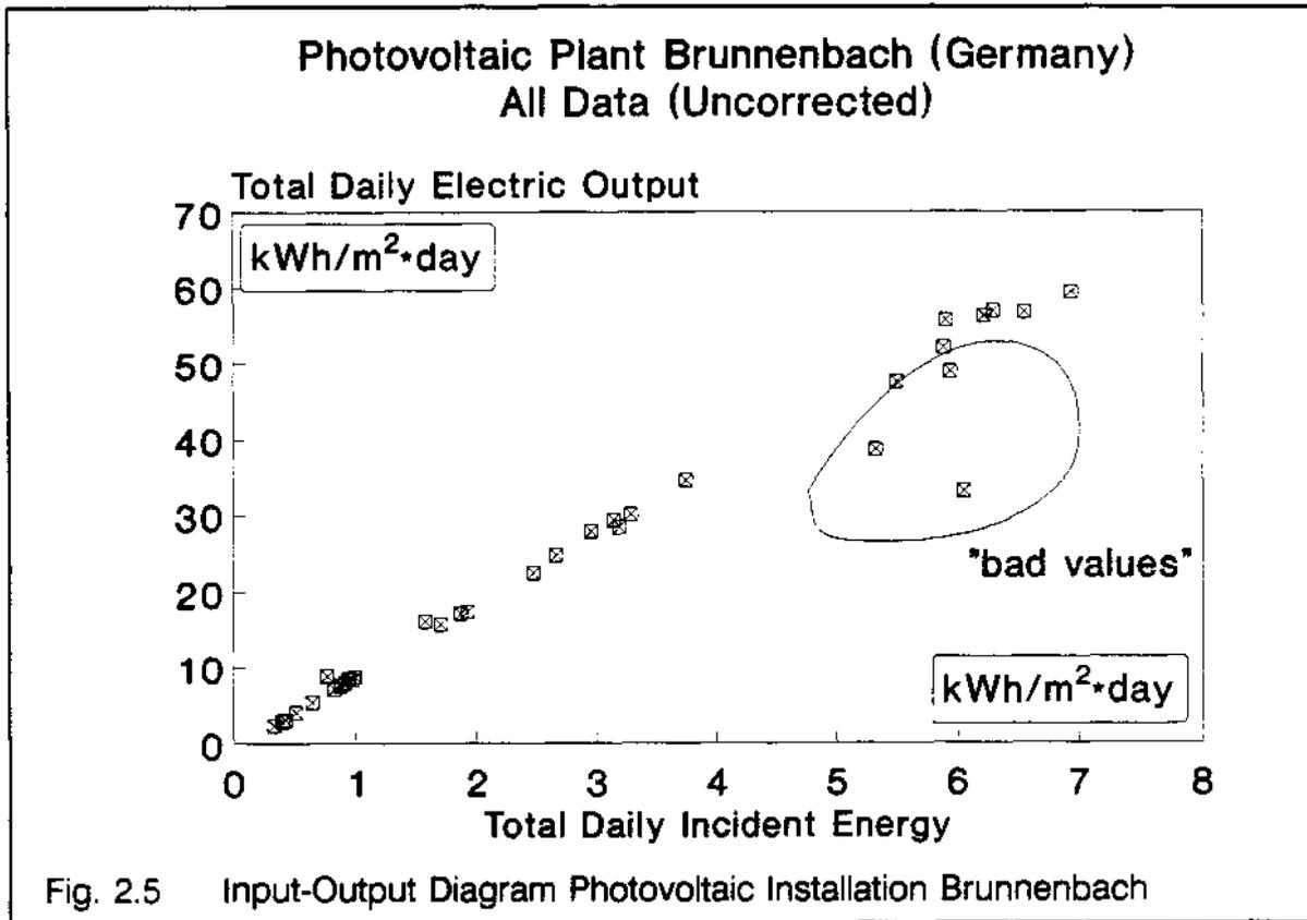
Fig. 2.5 Input-Output Diagram Photovoltaic Installation Brunnenbach
