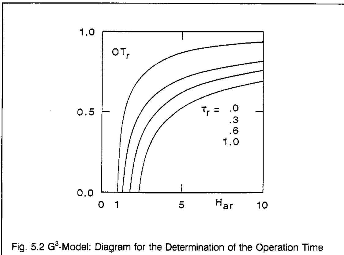
Fig. 5.2  $G^3$ -Model: Diagram for the Determination of the Operation Time
