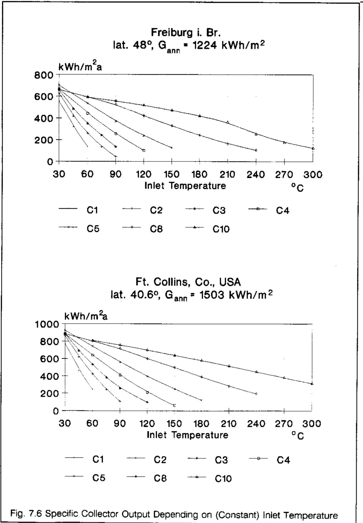
Fig. 7.6 Specific Collector Output Depending on (Constant) Inlet Temperature
