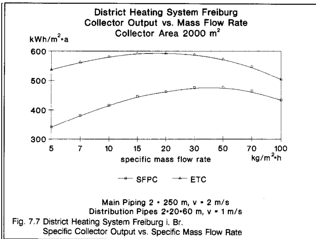
The specific collector output for different specific mass flow rates and inclinations is given in [fig 7.7](#) for Freiburg weather data. The optimum specific mass flow rates amount to approximately 40 kg/(m<sup>2</sup>\*h) for the selective flat plate collector and 20
