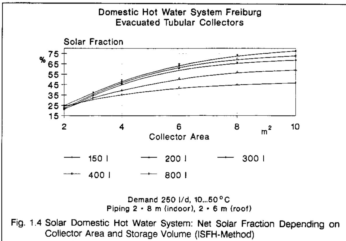
Fig. 1.4 Solar Domestic Hot Water System: Net Solar Fraction Depending on Collector Area and Storage Volume (ISFH-Method)
