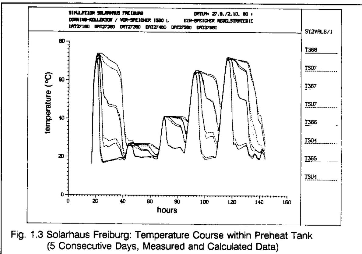
Fig. 1.3 Solarhaus Freiburg: Temperature Course within Preheat Tank (5 Consecutive Days, Measured and Calculated Data)
