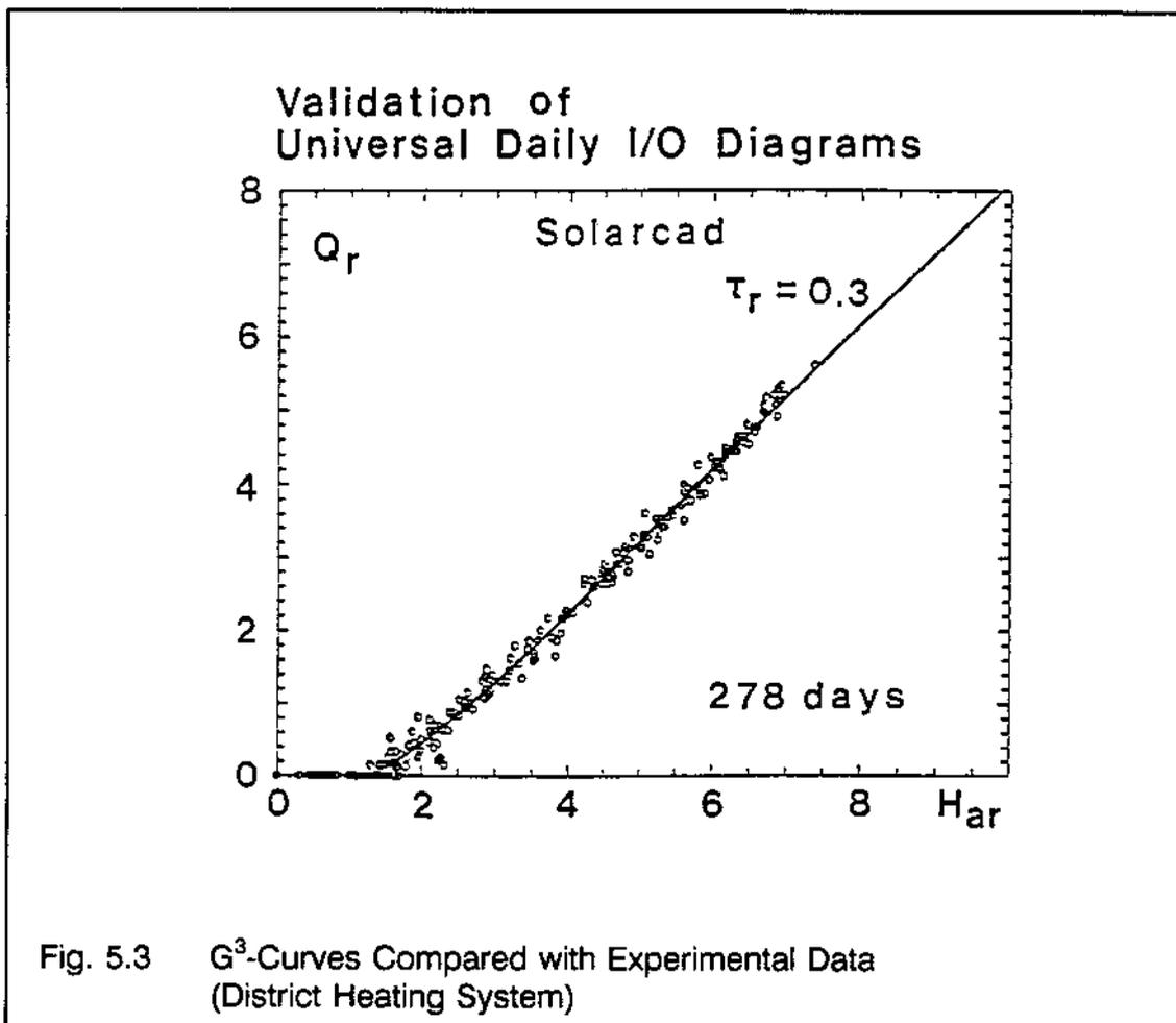
Fig. 5.3  $G^3$ -Curves Compared with Experimental Data (District Heating System)
