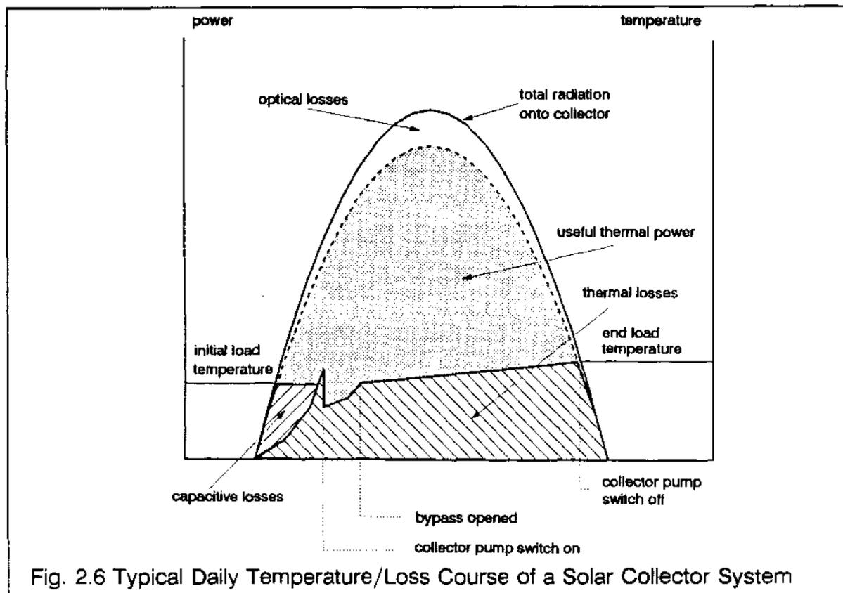
Fig. 2.6 Typical Daily Temperature/Loss Course of a Solar Collector System
